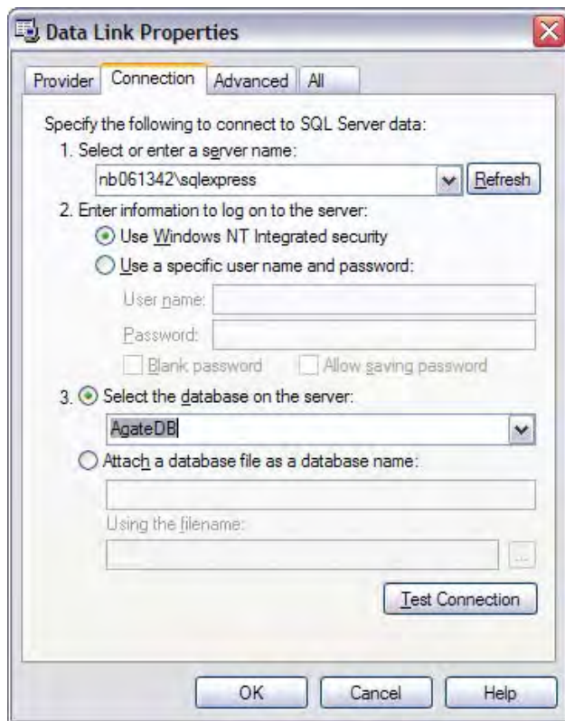
Fig. 4-5 Data linking server
