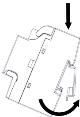
1. Place recesses of the device at the top edge of the mounting rail
