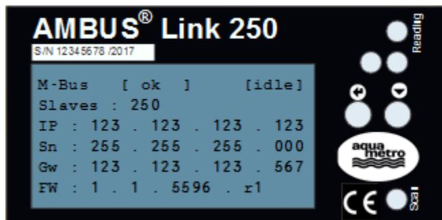
1. Hold the button for more than 2 sec. first position at IP is selected and configurable
