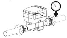
• Refer to the arrow on the side of the meter for the correct installation location (water must flow in the direction of the arrow).
