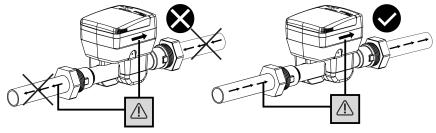
3. Remove old seals and clean sealing faces. The installation of the meter should not be done with force or strain, make sure that the meter is aligned.
