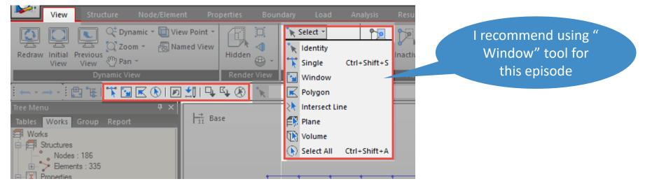
Tip #2: By clicking hidden, you can check graphics that reflect section shapes onto elements or element lines. Good tool to check for section properties locations!
