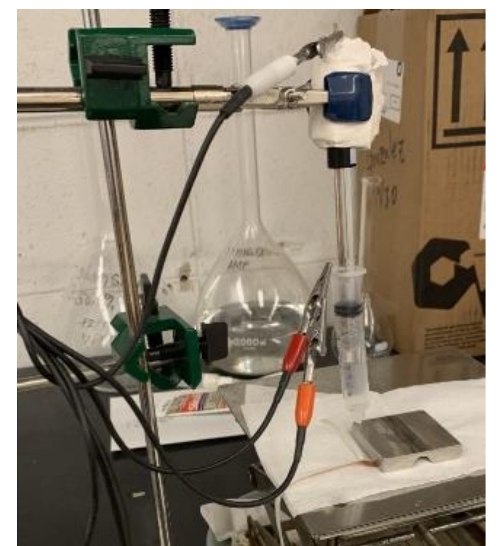
Electrochemical corrosion testing using syringe cell setup to determine the effect of non-backing gas welding on localized corrosion in the heat-affected zone (HAZ) and root weld metal.
