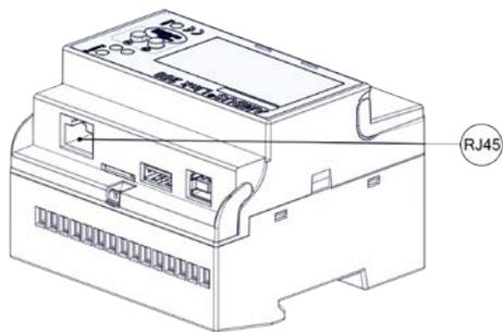
1. Plug the RJ-45 connector into the intended port
