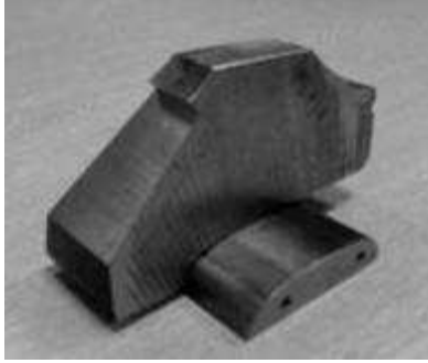
Figure 2. Photograph of the wheel and rail test specimen in contact.
