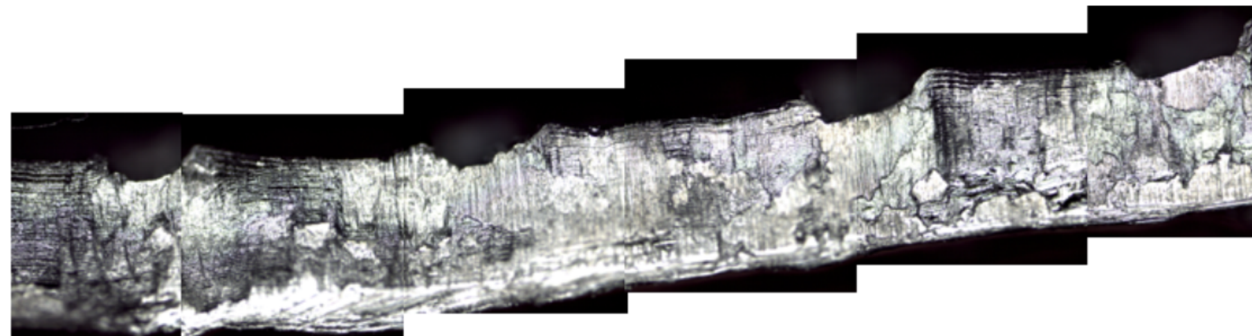
Cross section of the aluminum foil-to-foil weld, using a pneumatic based ultrasonic welding machine
