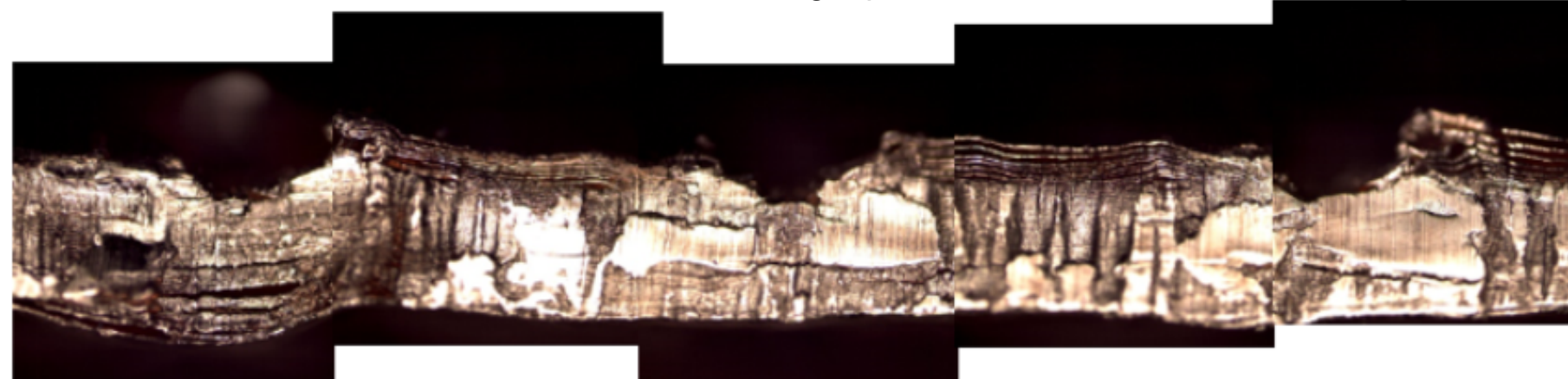
Cross section of the Copper foil-to-foil weld, using a pneumatic based ultrasonic welding machine
