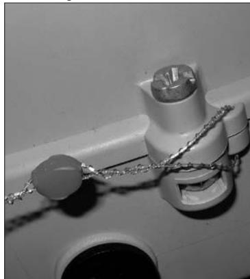
Seals on each of the two fixing screws of the measuring transducer
