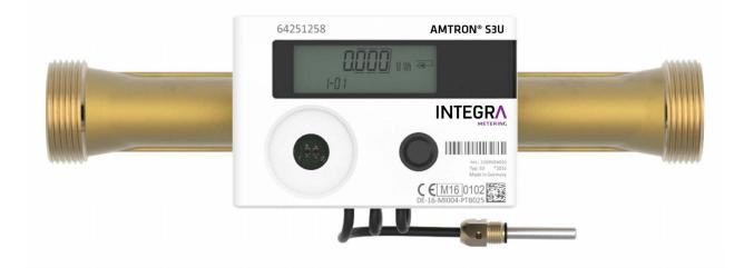
The compact meter AMTRON<sup>®</sup> S3U is used for heat and cooling measurements in small units, such as flats, offices and in local and district heating systems. AMTRON<sup>®</sup> S3U can be supplied with pulse output, M-Bus Interface or Wireless M-Bus (radio) according to the non-proprietary OMS<sup>®</sup> standard.
