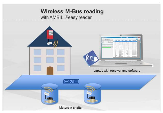
Example: AMBILL<sup>®</sup>easy reader for reading M-Bus/OMS wireless meters installed in an exposed location.
